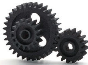
Picture taken after dye post-processing
